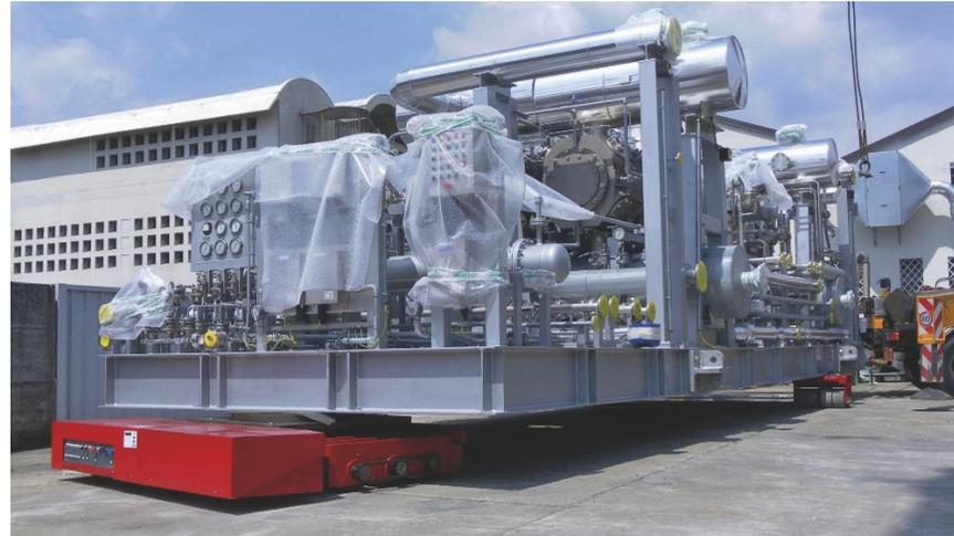
The self-propelled Dumbo trolley can lift and move loads from 20 to 200 tonnes.
